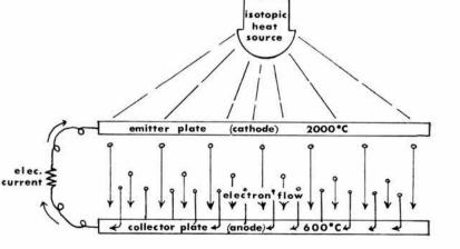
concept of using CVD rhenium to coat the electrodes. CVD rhenium forms in a preferred crystalline orientation and thus tends to emit or accept electrons more readily.
